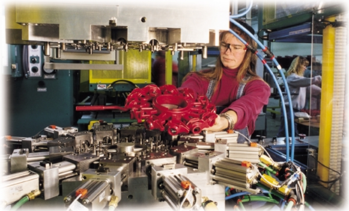
A multipart wax pattern is removed from a ring mold.
