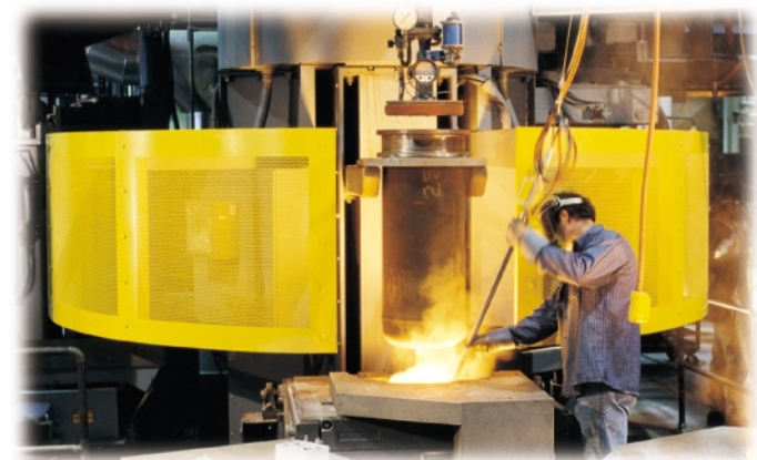
Hitchiner’s patented countergravity casting process.
