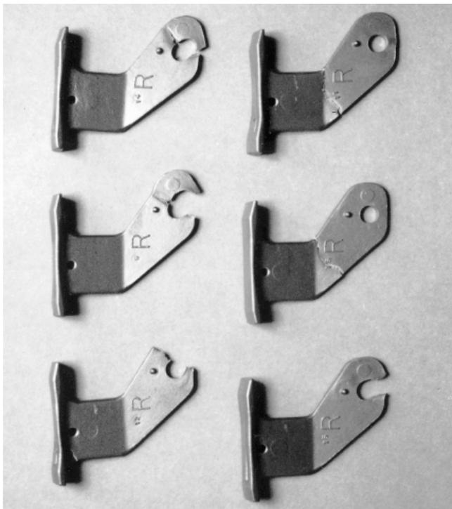
Figure 6. Seat belt slider parts in alloy 8630 that were tested to failure.
