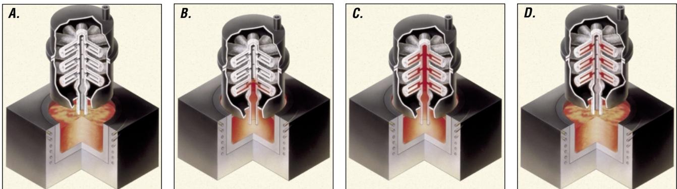
**Figure 1. The CLA process: A chamber that can be closed and sealed holds a permeable mold; an open, impermeable fill pipe extends out of the chamber, (a). The fill pipe lowers into the melt and an applied vacuum draws molten metal, (b), up into the mold in a highly controlled fashion. Castings solidify while the passage stays molten, (c). When the vacuum releases, most of the gating metal returns to the melt for reuse and the castings are all separate in the mold, (d).**
