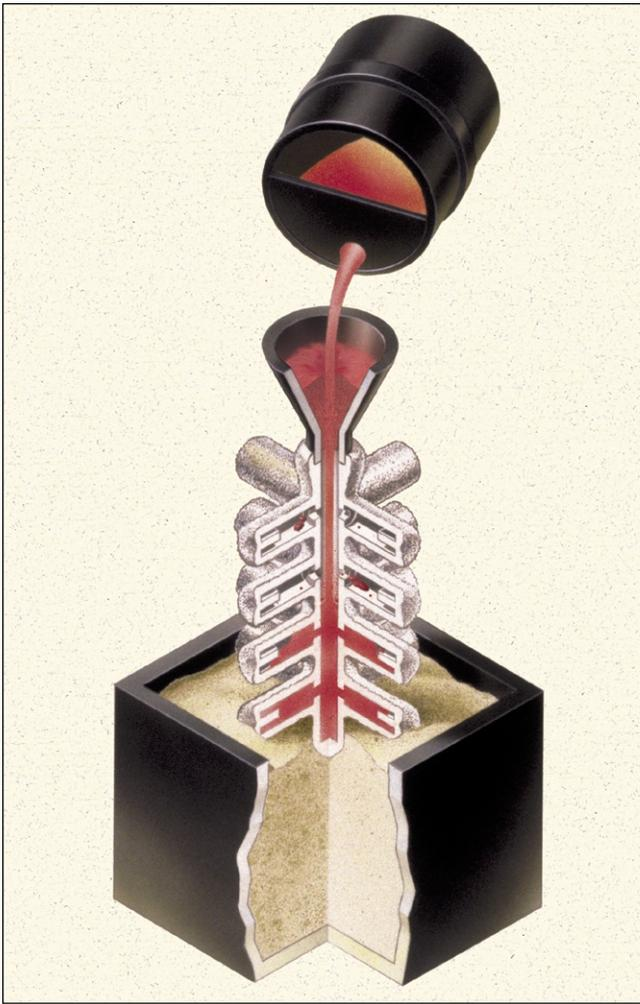
**Figure 2. Conventional gravity pouring:** The metal swirls in the pour cup, splashing sideways to splatter metal into upper cavities, and falls to the bottom, splashing metal into many cavities at once. The bottom cavities do not fill until the central passage builds up enough height (pressure) to force the air out of the lower cavities. Variation in filling from part to part in a mold is great.
