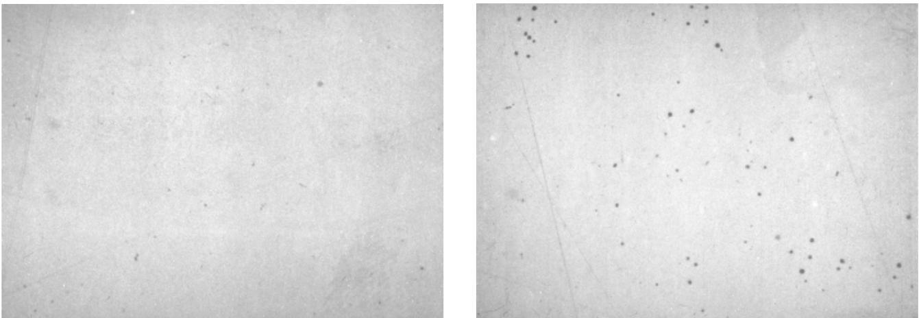
**Figure 4. CLA cast cleanliness, left, vs. gravity cast, right, for 17-4PH stainless steel. Other alloys also show CLA metal cleanliness to be superior.**
