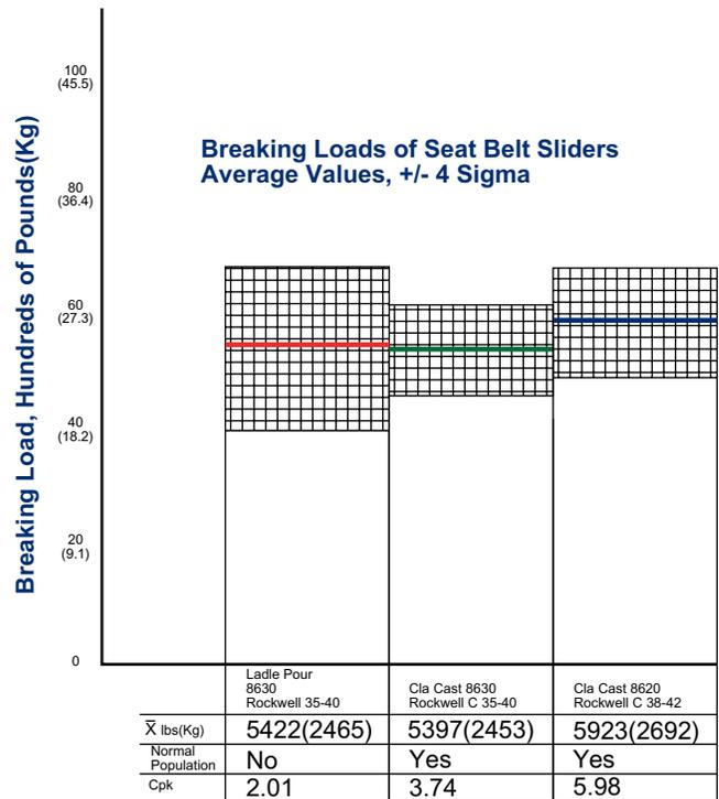
Figure 7. Comparison breaking loads of ladle-poured and CLA-cast seat belt sliders.
