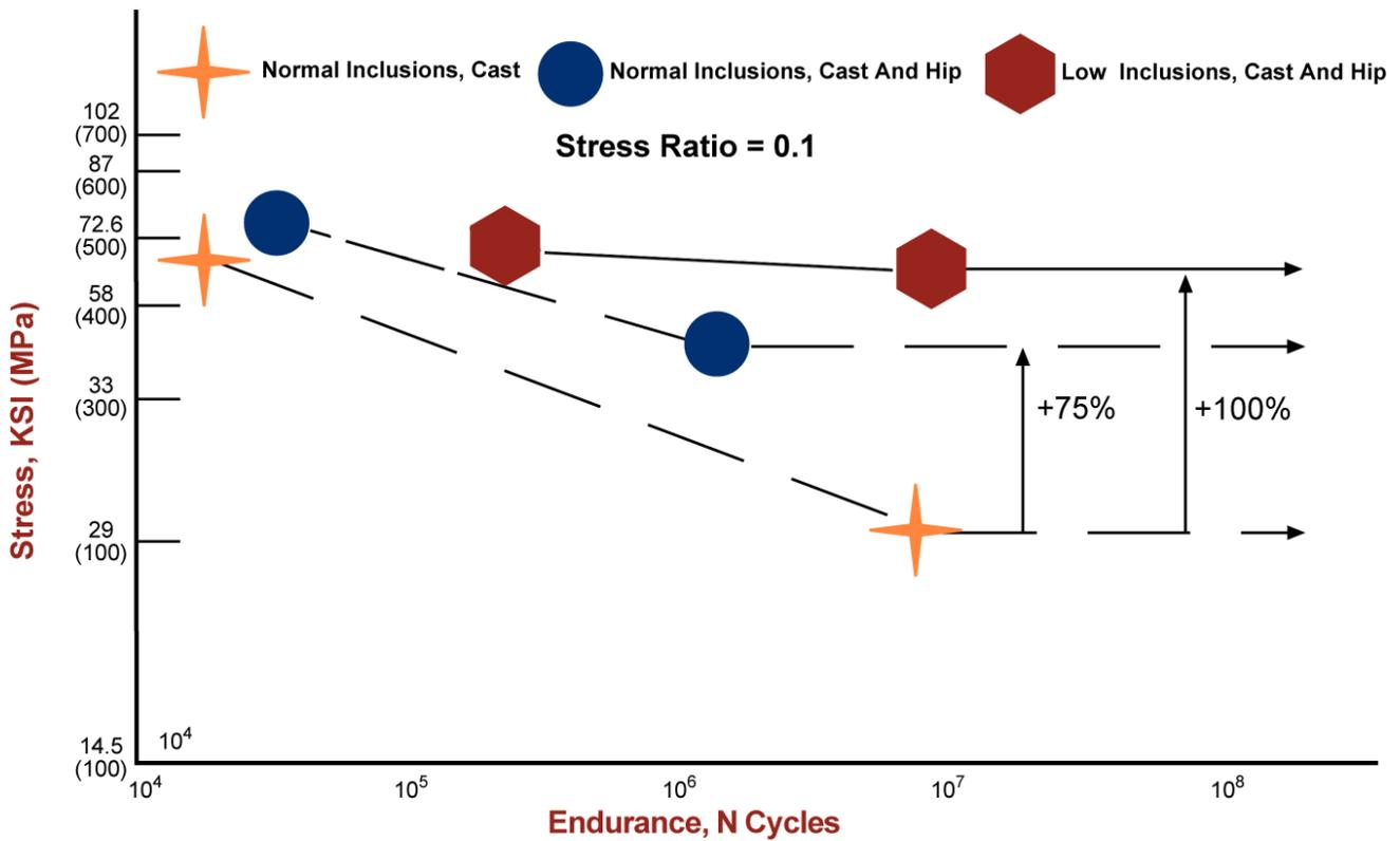
Figure 5. These stress/number of cycle curves for 17-4PH stainless steel show the great importance of microporosity closed by hot isostatic pressing and the presence of inclusions eliminated by vacuum casting.
