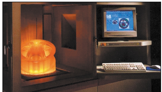
Figure 2. SLA-7000 rapid prototyping system used by Brookfield Rapid Solutions to produce prototype casting patterns for Hitchiner and its customers.
