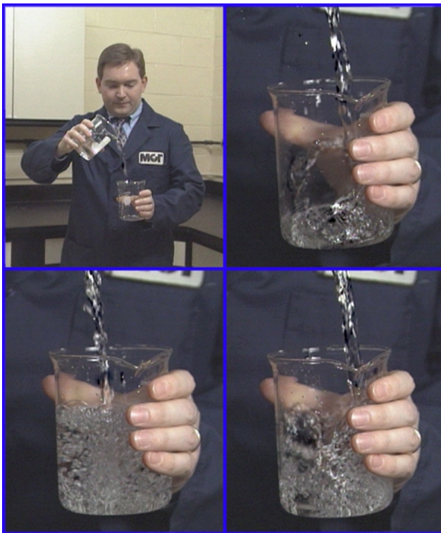
Figure 1. Water poured into a beaker (clockwise from top left) generates dozens of bubbles. When casting metals by gravity pouring, such bubbles collapse, leaving oxide defects in the casting.
