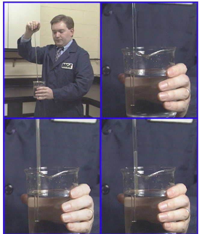
Figure 2. Water vacuumed upward into a container is bubble-free (clockwise from top left). When metal is cast this way, the resulting casting typically contains only about 15% of the oxides found in poured castings.
