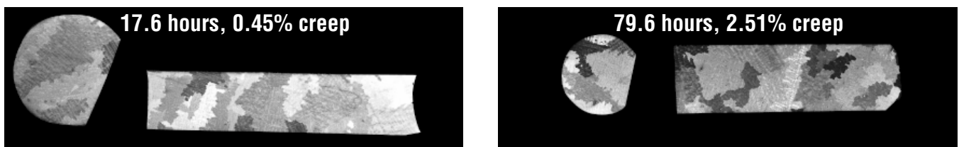
Figure 4. Two bars machined from the same blade side-by-side to eliminate many variables. Note the grain structure at the fracture area. The bar with the finer grain at fracture is clearly better. (2.6X)
