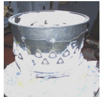
Figure 3. Diffuser case CLI-cast in Inco 718 alloy. The CLI cast diffuser case measured 35 inches (899 mm) in diameter and 25 inches (635mm) in height.
