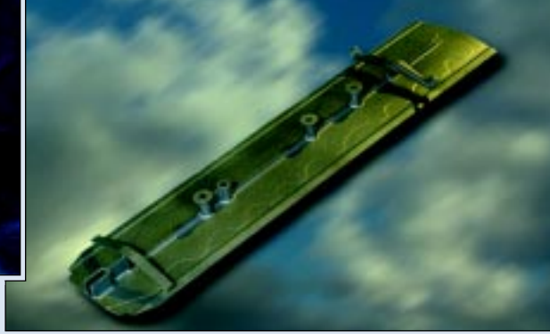
The Gas Turbine Div. follows a traditional approach to wax pattern building for its thin-walled jet engine castings such as this jet engine after-burner seal. However, the CLV counter-gravity process for vacuum alloys allows it to produce the defect-free, thin-walls required for aerospace applications.
