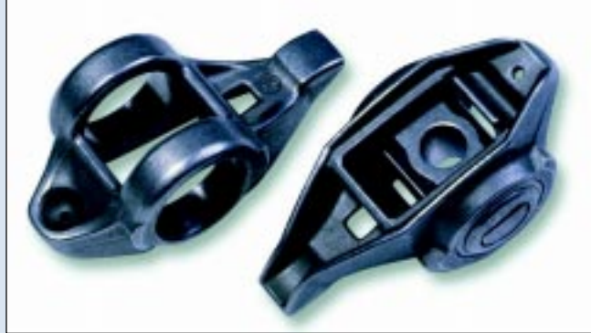
Fig. 2. These Chevrolet steel roller rocker arms were produced by Hitchiner's Mexico Div. Rocker arm production represents Hitchiner's "push of the casting envelope" as the foundry turned a stamping into a casting and improved the part's strength, complexity and functionality via counter-gravity casting.
