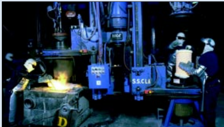
Hitchiner's SSCLA counter-gravity casting process produces steel roller rocker arms at the Mexico Div. The SSCLA process uses a ceramic shell mold with fewer layers, which is backfilled or supported by sand before undergoing counter-gravity casting.
