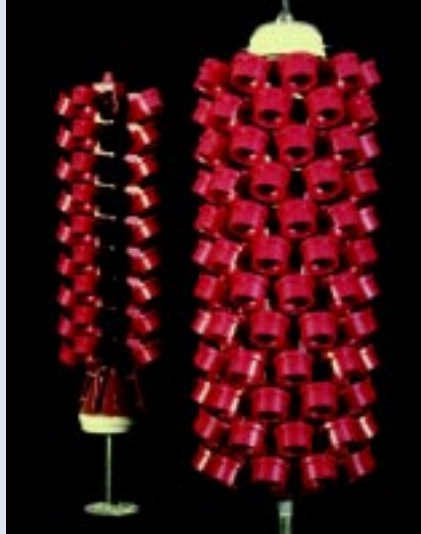
Fig. 1. A benefit of counter-gravity casting is the amount of patterns attached per investment tree. The Hitchiner investment tree (r) holds up to five times as many castings as the traditional tree.
